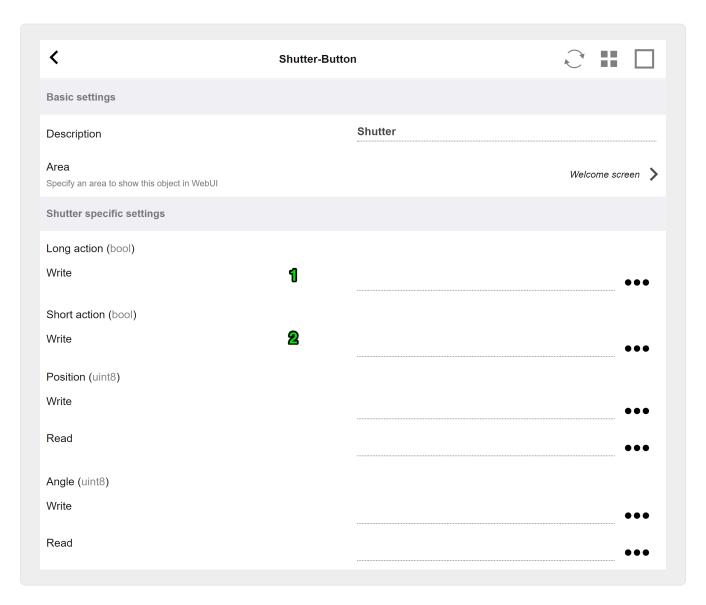
Most important with a KNX shutter actuator are the long action (1) to drive it fully up or down, and short actions (2) to change the slat angle. Direct writing of Position and Angle as an 8-bit value may be supported only by some KNX actuators.
