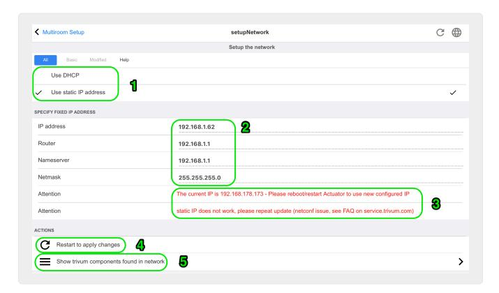
trivum multiroom devices support static and dynamic IPv4 IP addresses (over DHCP router). For smooth interaction between all trivum devices in your network, we recommend the use of DHCP.
