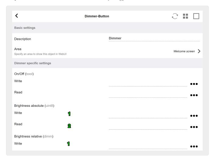
the dimmer is a binary actuator, extended by fields to set (1) or read (2) brightness.
