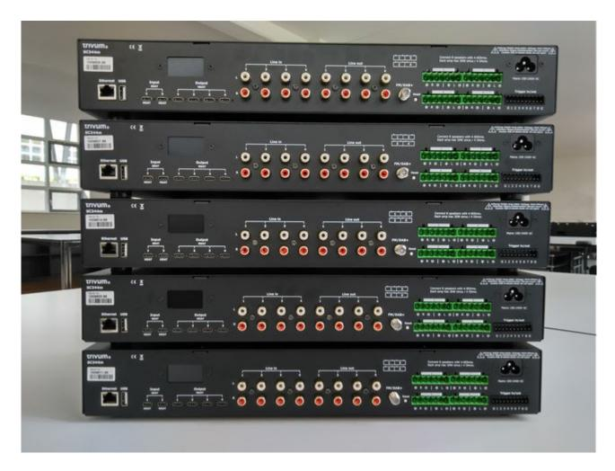
Select which device should be master, in this example the topmost. Change all other devices to slave mode:
