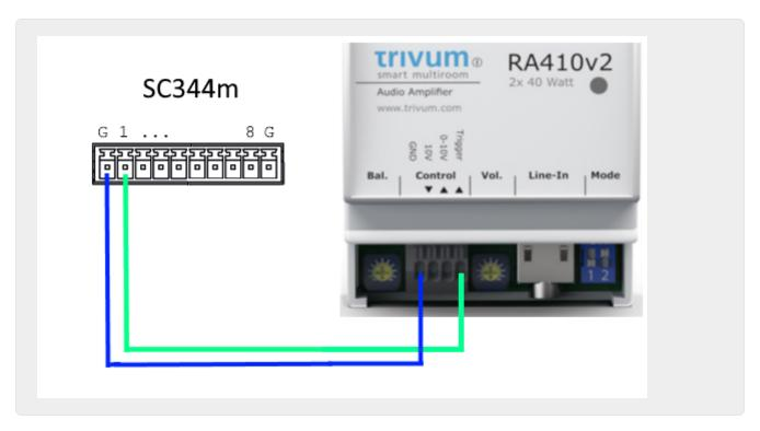
Example how to connect output 1 triggering to an old RA410v1 amplifier, in stereo mode. Note that On A and On B on amplifier side are short-circuited, to tell the amplifier it should run in stereo mode. This way only 2 control wires are needed from the SC to the amp.
